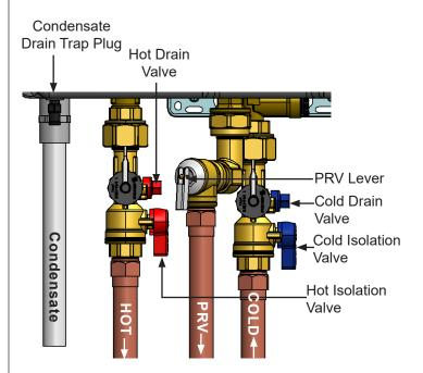
Figure 79: Piping Diagram
