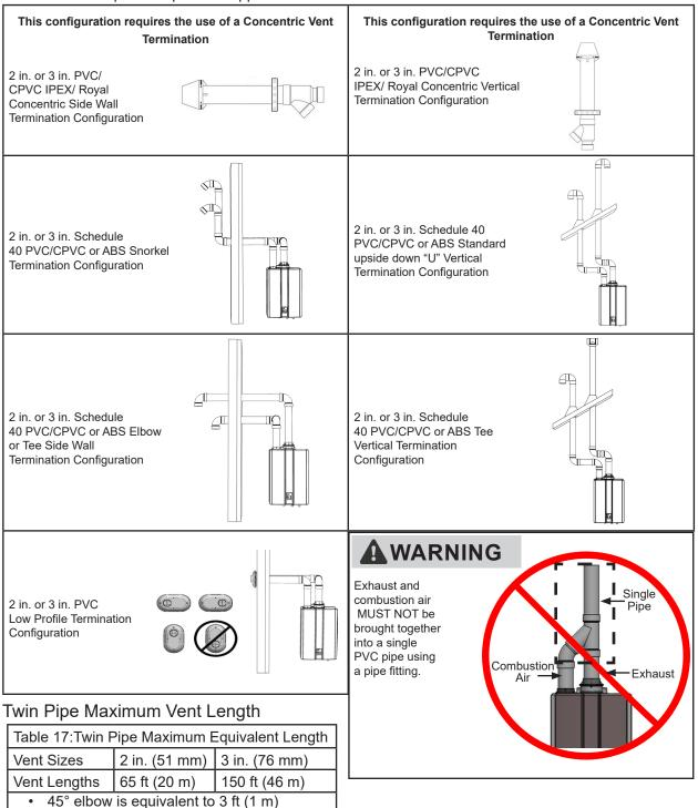
• 90° elbow is equivalent to 6 ft (2 m)
