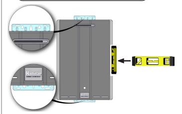
Figure 13: Mount water heater
