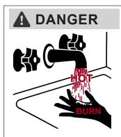
Water temperatures over 125°F (52°C) can cause severe burns or scalding resulting in death.
