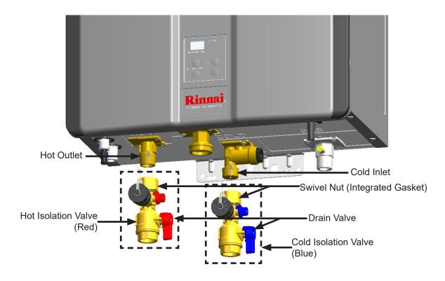
Figure 52: Install Isolation Valves
