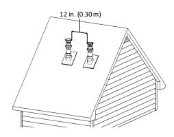
Figure 25: Between terminals at same level
