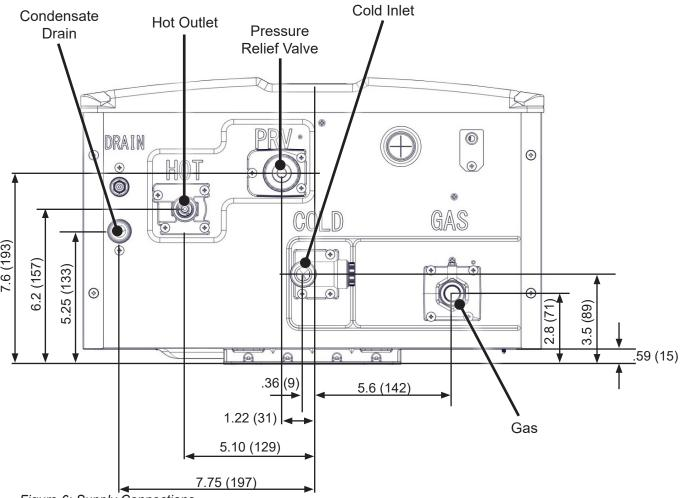
Figure 6: Supply Connections
