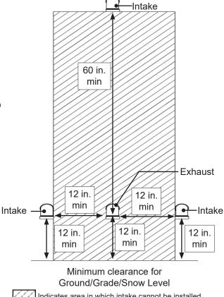
Indicates area in which intake cannot be installed.
