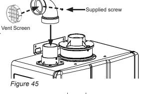
Install the exhaust vent pipe. Ensure it is properly seated.
