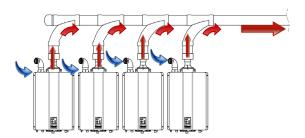
Figure 20: Common Vent, Room Air
