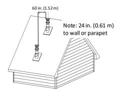
Figure 24: Between terminals at different levels
