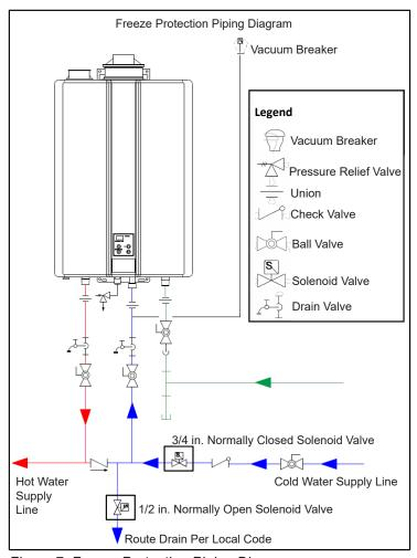
Figure 7: Freeze Protection Piping Diagram
