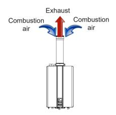
Figure 23: Concentric Pipe
