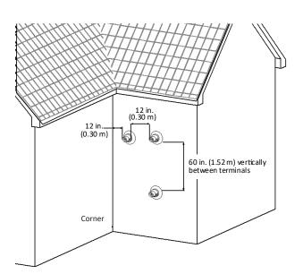
Figure 22: Concentric Pipe Termination Clearances
