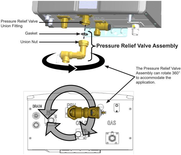
Figure 53: Pressure Relief Valve Assembly
